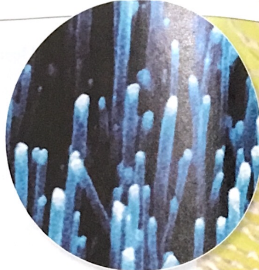
The carbon nanotubes shown growing in the picture above have been magnified 295 times.
