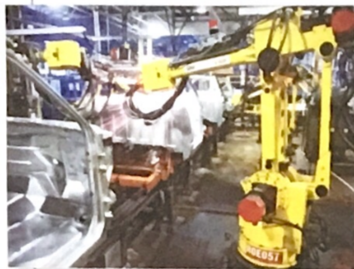
The elbow of this welding robot allows the welding torch to be handled in almost the same ways in which a human would handle it.
