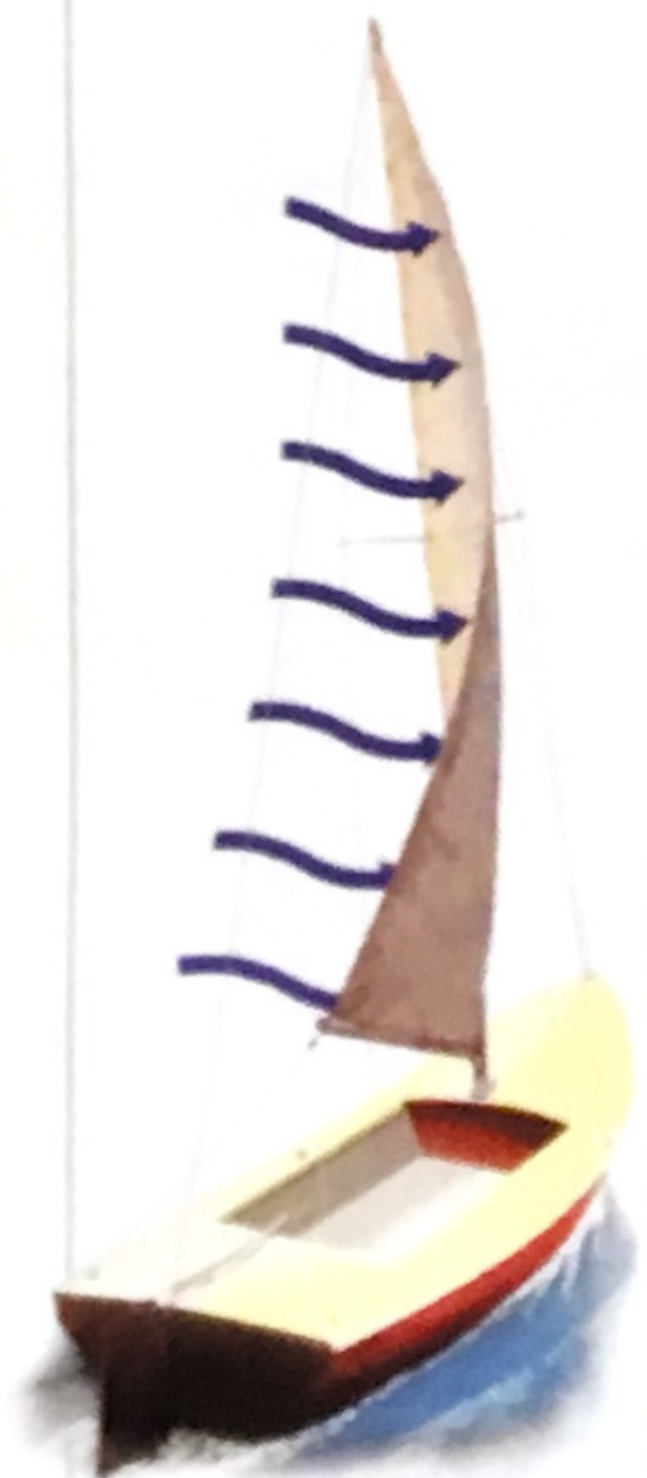
The force of the wind against the sail causes a sailboat to move through water. By rotating the sail, the sailboat's direction of motion can be changed.
